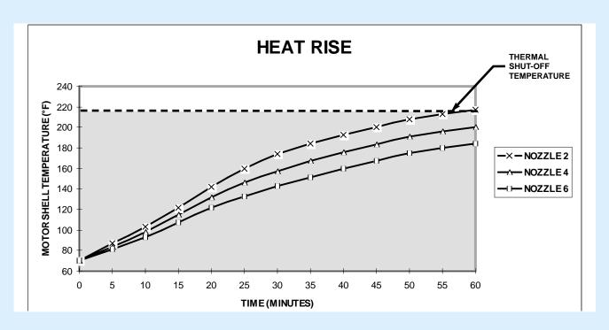
The motor driving this pump has a built in thermal protector that will open, shutting off the pump, when the surface temperature of the motor heats to approximately 215°F. Motors of this size and construction require 15 to 30 minutes of cooling time before the thermal protector closes and re-energizes the pump. Lower current levels heat more slowly, allowing longer run times, but the cool down time still averages about 30 minutes, at 70°F ambient temperature.
